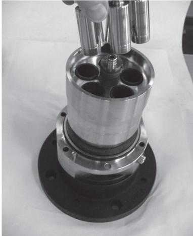
21. Position the housing on the port flange and over the guide pin.
