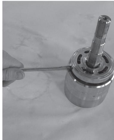
10. Replace the O-rings and the back-up rings on the valve plate. Mount the new back-up rings on the new valve plate first and then mount the new O-rings.
