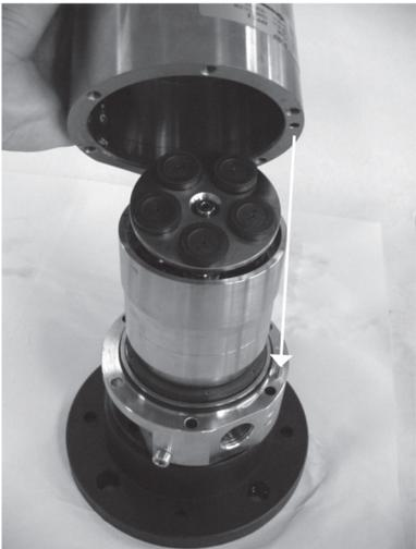
22. Hold the pump together and carefully turn it over to rest on the housing. To prevent seizing-up, lubricate the threads on the 2 screws and screw them into the port flange and the housing. Use Molykote D paste from Dow Corning or Klüber UH1 84-201 from Klüber Lubrication. Tighten the 2 flange screws to a torque of 12+1Nm.
