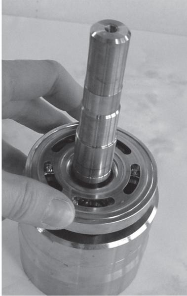
13. Gently push flushing valve out using the Allen key.
