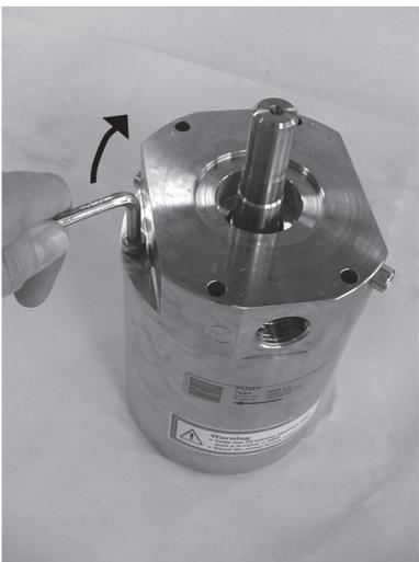
23. Mount the new shaft seal following the instructions in changing "Shaft seal - APP 1.5 - 2.5" (180R9089)
