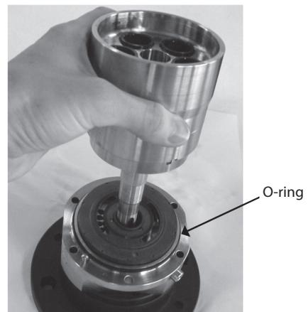
20. Position the new spring, new spring guide, new retainer guide, new retainer plate and new pistons.
